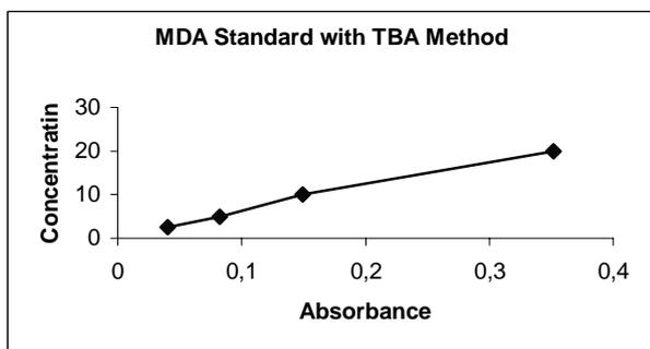
**Figure 3.** MDA standard curve used for TBA method, prepared in the same condition with the sample
