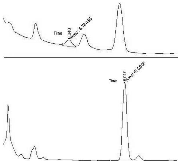
**Figure 5.** HPLC chromatograms of liver total MDA deproteinized with acetonitrile after DNPH derivatization with and without added standard (20 µl injected) column ODS2 C18 reverse phase (125x4.6mm) mobile phase: acetonitrile-distilled water. Sample preparation is as described in the text. a) Control liver, b) Control liver + added standard
