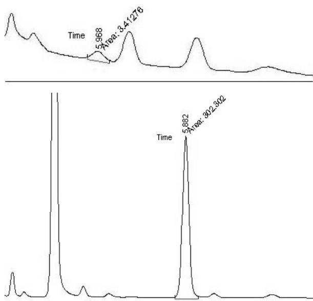
**Figure 6.** HPLC chromatograms of kidney total MDA deproteinized with acetonitrile after DNPH derivatization with and without added standard (20 µl injected) column ODS2 C18 reverse phase (125x4.6mm) mobile phase: acetonitrile-distilled water. Sample preparation is as described in the text.
