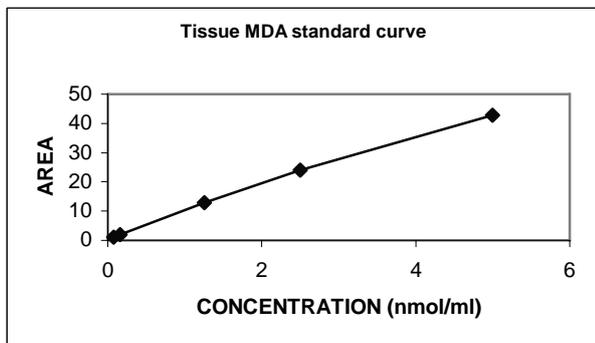
**Figure 2.** Tissue MDA standard curve, with regression line, prepared in the same condition with sample (filtered before HPLC)
