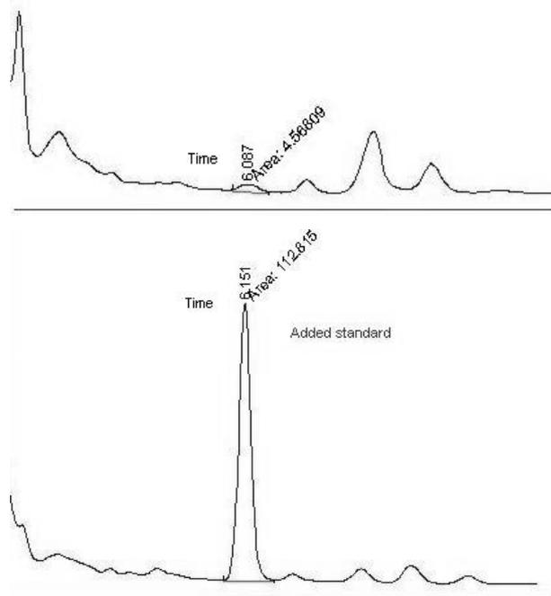
**Figure 4.** HPLC chromatograms of plasma total MDA after DNPH derivatization with and without added standard (20 µl injected) column ODS2 C18 reverse phase (125x4.6mm) mobile phase: acetonitrile-distilled water. Sample preparation is as described in the text.
