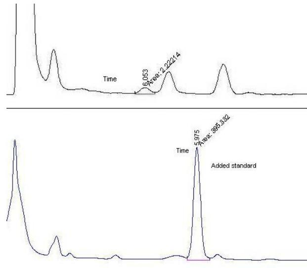
**Figure 7.** HPLC chromatograms of brain total MDA deproteinized with acetonitrile after DNPH derivatization with and without added standard (20 µl injected) column ODS2 C18 reverse phase (125x4.6mm) mobile phase: acetonitrile-distilled water. Sample preparation is as described in the text.
