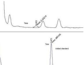
**Figure 7.** HPLC chromatograms of brain total MDA deproteinized with acetonitrile after DNPH derivatization with and without added standard (20  $\mu$ l injected) column ODS2 C18 reverse phase (125x4.6mm) mobile phase: acetonitrile-distilled water. Sample preparation is as described in the text. a) Control brain
