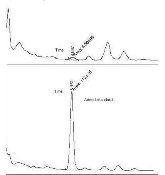
**Figure 4.** HPLC chromatograms of plasma total MDA after DNPH derivatization with and without added standard (20  $\mu$ l injected) column ODS2 C18 reverse phase (125x4.6mm) mobile phase: acetonitrile-distilled water. Sample preparation is as described in the text.
