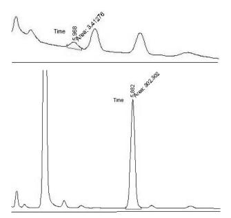
**Figure 6.** HPLC chromatograms of kidney total MDA deproteinized with acetonitrile after DNPH derivatization with and without added standard (20  $\mu$ l injected) column ODS2 C18 reverse phase (125x4.6mm) mobile phase: acetonitrile-distilled water. Sample preparation is as described in the text. a) Control renal cortex
