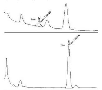
**Figure 5.** HPLC chromatograms of liver total MDA deproteinized with acetonitrile after DNPH derivatization with and without added standard (20  $\mu$ l injected) column ODS2 C18 reverse phase (125x4.6mm) mobile phase: acetonitrile-distilled water. Sample preparation is as described in the text. a) Control liver, b) Control liver + added standard
